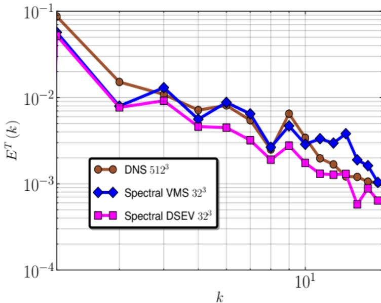
The VMS-based model performs very well. The dynamic Smagorinsky model is overly dissipative.
